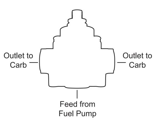
Adjustable non bypass fuel pressure regulator for mechanical or low pressure inline fuel pumps. All fittings are 3/8" NPT. One outlet may be plugged off for single feed applications.
